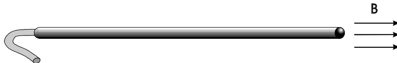
Fig. 7: Positive Field Direction for Axial Probe
