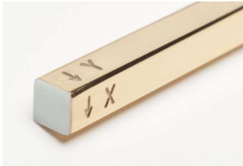
Figure 4 marking of measurement direction on the probe
