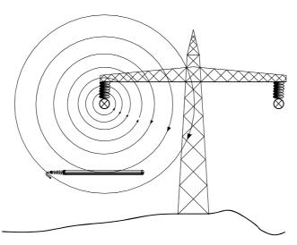
Figure 5: Field of a single high voltage line
