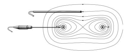
Figure 6: Field with two conductors (rectified currents)
