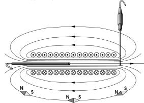
Figure 2: Cylindrical inductor
