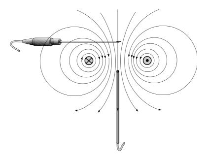
Figure 7: Field with two conductors (opposing currents)
