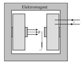
Figure 12: Electromagnet with probe for field control
