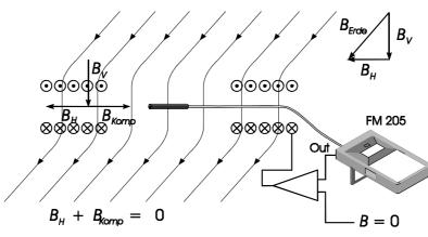
Figure 11: Compensation of the Earth's magnetic field
