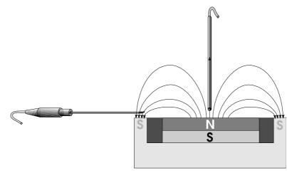
Figure 8: Holding magnet disc
