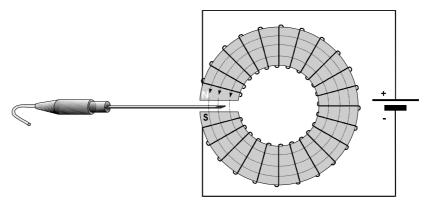
Figure 3: Electromagnet
