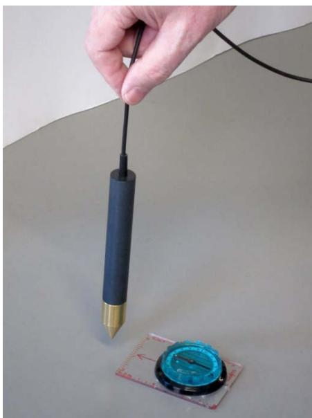
For measuring the vertical component of the Earth's magnetic field, on the other hand, the probe AS UAP Lot offers itself. This can be used hanging like a solder on the cable.
