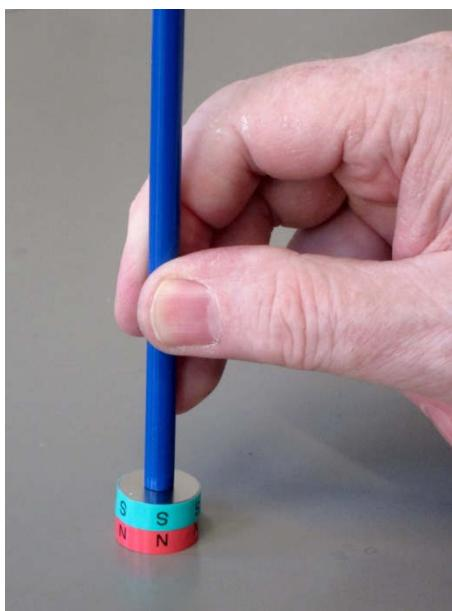
In contrast, the axial probes are placed perpendicular to the magnet for measurement, since this probe measures only the field component parallel to the probe.
