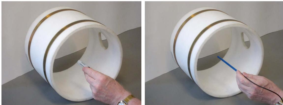
Since the interior space is accessible from the side between the two coils, it is also possible to measure with a transversal probe. If the coil diameter is large enough, it is also possible to place the probe inside the coil.
