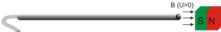
If a transversal probe is now placed with the cross up on a magnet or if the axial probes are mounted vertically on a magnet and the teslameter shows a positive value, then there is a south pole underneath the probe. If a negative value is displayed, it is the north pole.
