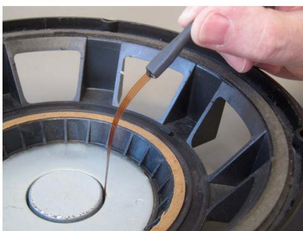
Even thinner and, moreover, even more flexible is the probe AS-NTP Flex, which can thus be used, for example, in suitable for measuring in air gaps of loudspeakers.
