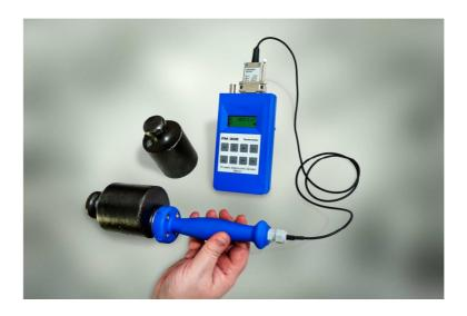
Especially for these measurements, together with the State Office for Metrology and Calibration Berlin-Brandenburg, we have developed a handle for the AS-LAP probe. The handle is provided on its underside with a protective plate made of aluminum.
