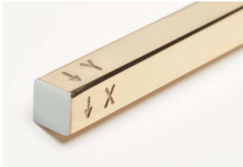
Figure 4 marking of measurement direction on the probe
