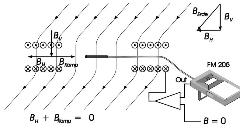
Figure 2 Compensation of an external magnetic field
