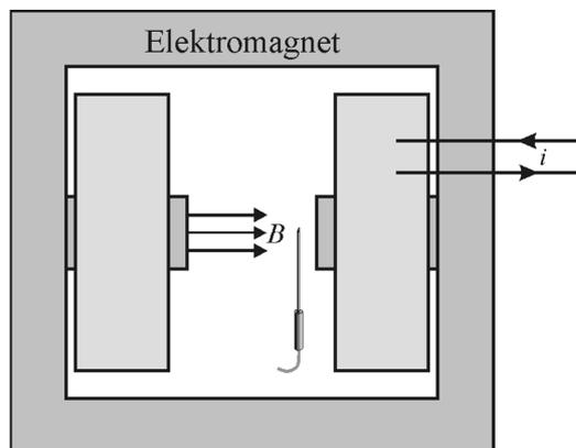
Figure 1 Electromagnet with probe for field control
